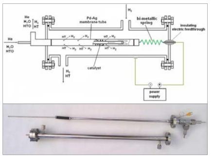
**Fig.1** Scheme (top) and picture (botton) of a Pd-membrane reactor for the recovering of tritium from tritiated water via isotopic exchange. Fig. 1 (top) reprinted from [5], with permission from Elsevier.
