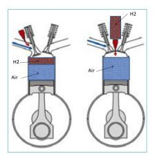
Fig.1 intake fuel injection and direct injection of H<sup>2</sup> in ICE
