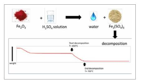
Fig.4 Alternative decomposition of sulfuric acid: the acid concentrated solution is reacted with Iron(III) oxide obtaining Iron(III) sulphate. The latter, as illustrated in the thermogravimetric pattern on the bottom, decomposes into Iron(III) oxide, sulphur oxides and oxygen at a lower temperature level than  $H_2SO_4$  itself (between 650°C and 700°C).
