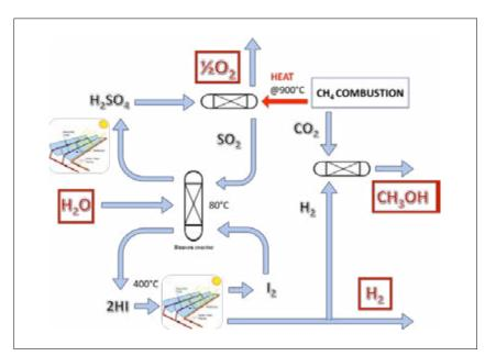
Fig.3 Alternative of the "Sulphur Iodine" scheme where  $H_2SO_4$  cracking is driven by methane combustion. The obtained  $CO_2$  is reacted with part of the produced  $H_2$  in order to synthetize methanol.
