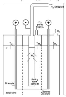
Fig.4 Alkaline electrolyser with Pd-Ag thin-wall tube acting as cathode. Reprinted from [15], with permission from Elsevier
