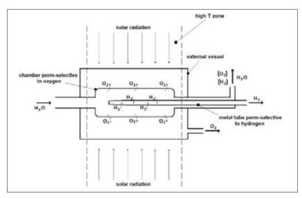
Fig.6 Schematic configuration a solar-powered membrane reactor. Reprinted from [20].
