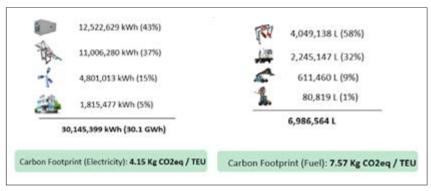
Fig.4 Energy Profile of Container Terminals. Electrical and Fuel Consumption [3].
