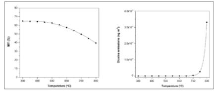
**Fig.5** Methane yield (left) and dioxins emission (right) of a hydrogasification reactor fed with 1000 kg <sup>h-1</sup> of dry RDF and a hydrogen excess of about 40 kg h<sup>-1</sup>. Reprinted from [18], with permission of Elsevier.
