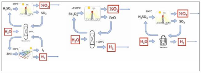
Fig.1 Three widely studied TWSCs: a) "Sulphur Iodine" b) "Iron Oxide" and c) "hybrid sulphur" cycles
