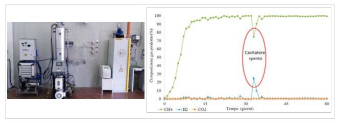
Fig.1 Hydrogenotrophic methanogenic reactor (1a - image on the left) and outlet gas composition (1b - chart on the right).
