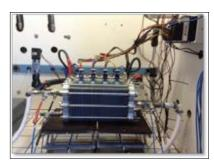
**Fig.1** CNR ITAE-developed polymer electrolyte fuel cell stack prototype under laboratory testing.
