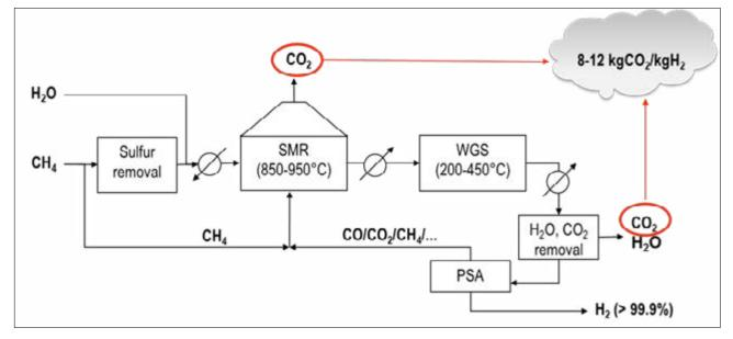
Fig.1 General scheme of a conventional steam methane reforming process
