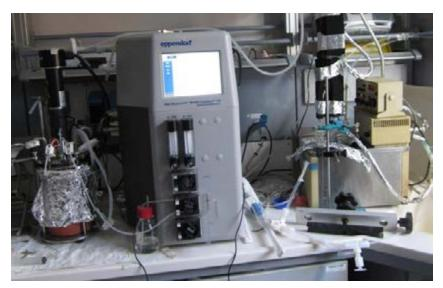
$\ensuremath{\mathsf{Fig.2}}$  GRAIL project: 3L biofermenter collected to the gas-stripping apparatus for ethanol collection
