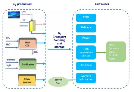
Fig.1 simplified scheme of hydrogen implementation in different industry sector
