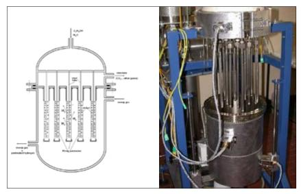
Fig.3 Scheme (top) and picture (botton) of a multi-tube membrane reactor for the production of hydrogen via ethanol steam reforming. Fig. 3 (bottom) reprinted from [4], with permission from Elsevier.
