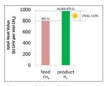
Fig.3 Energy balance of solar steam methane reforming process in the solar fuel perspective
