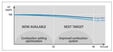
**Fig.2** Engine derating to fulfill NOx emission limitations, taken from ANSALDO ENERGIA [9].
