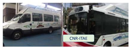
Fig.4 CNR-ITAE hydrogen fuel cell city buses under testing on urban paths (I-NEXT, H-bus projects).
