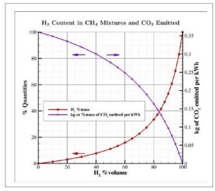
**Fig.1** Relation between volume and mass percentages in methane/hydrogen mixtures, and impact in terms of CO<sup>2</sup> emitted (assuming an electrical efficiency of 55%). The percentage quantities on the left are with respect to pure methane.
