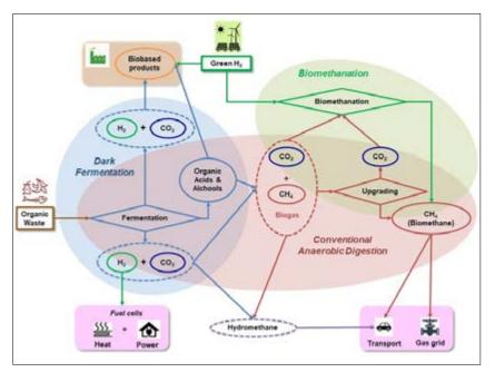
**Fig.1** Biological processes integrated in the green H2 value chain: Background coloured areas enclose the main step of each process; Rectangles represent process; feeding Diamond shapes represent technological stages; Round shapes represent products; Dotted lines enclose gas mixtures; Background coloured rectangles represent the end uses.
